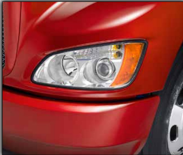
An advanced forward lighting system provides up to 30% more down-road coverage than conventional sealed beam designs. Choose the standard halogen or optional HID Xenon lamps.
