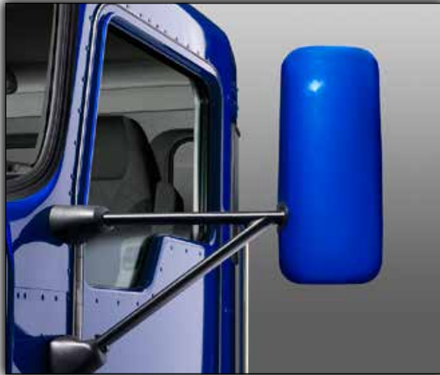
Heated and electronically-adjusted aerodynamic mirrors are cowl mounted to reduce vibration and readjustment.
