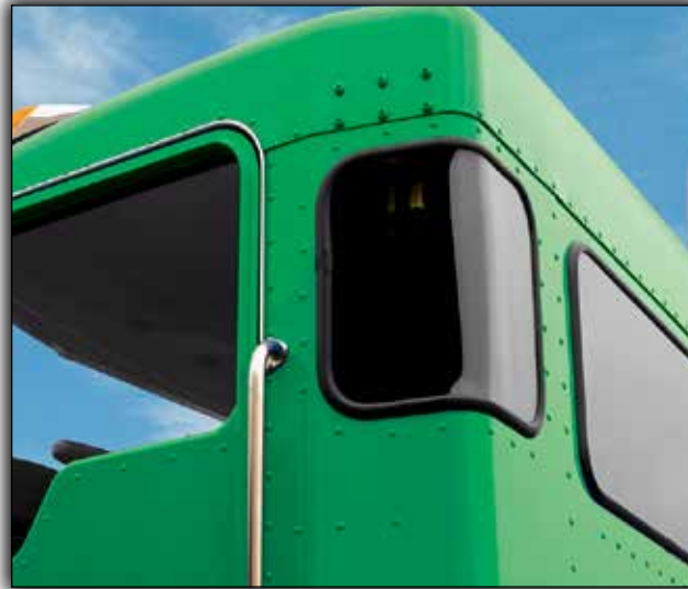
In addition to the standard peeper window in the passenger door, optional cab corner windows are available to help improve visibility in tight places.
